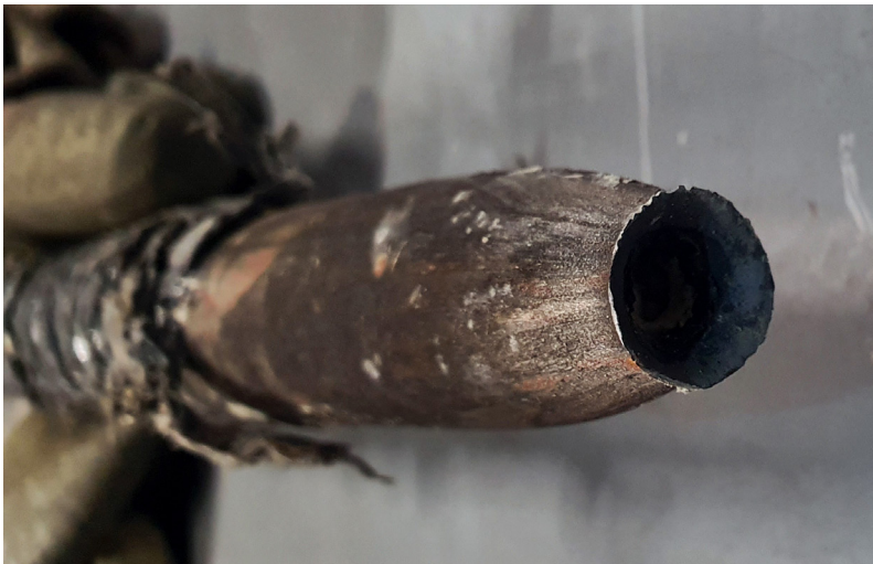
Figure 4. The bonding capacity of mineral bolt resin allows full utilisation of steel ductility.
