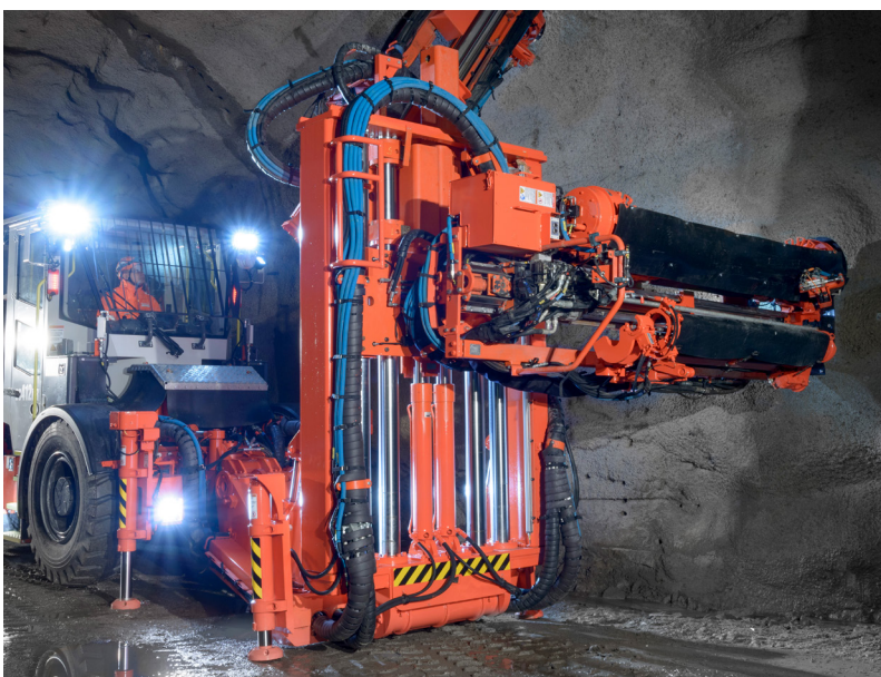
Figure 5. Sandvik DS412i-R is equipped with a double bolting turret and complete injectable resin systems, ready for hollow bar/self-drilling anchors.
